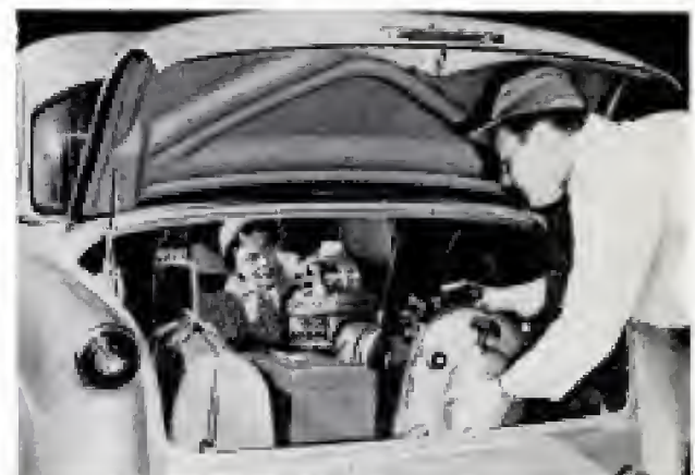
HUDSON Jet has a removable rear seat. With it out, trunk divider wall drops to make huge loading area
